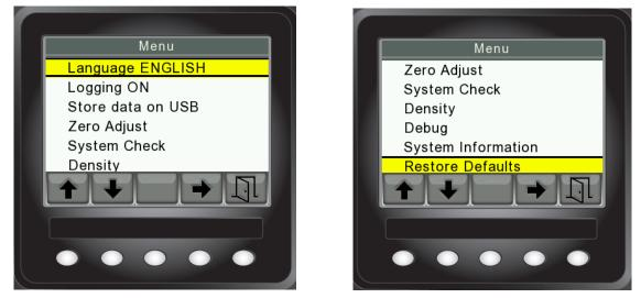
Vertical arrow buttons scrolls up and down in the menu. Horizontal arrow button selects the highlighted function, and switches between ON/OFF. Rightmost button (open door) Returns to previous view.
