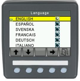
Choose the desired language by pushing the vertical arrow buttons. After pressing the horizontal arrow button, to select the Language, and then the door symbol, the next setting will appear on the display screen.
