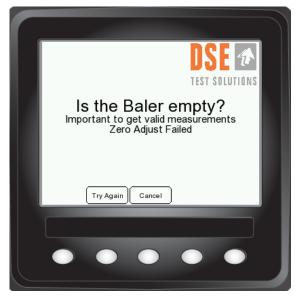
The most likely source of error is missing connection to the TX or RX units, material in the baler or similar disturbance of the measurement.
