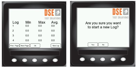
The New Log button adds a new log number to the list. As it is not possible to go back to an older Log and continue adding to it, the user is asked to confirm the creation of a new log number.
