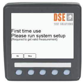
Selections are made by pressing the corresponding push button below the "button" on the screen.
