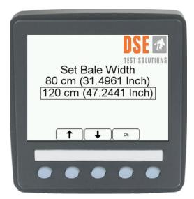
After choosing the Bale Width appropriate to the baler and pushing the Ok button, the next image will appear on the display screen.
