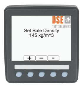
Set the correct Bale Density with the + and – buttons. Push the Ok button, for next setting.
