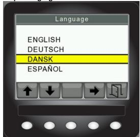
Select language by using the up/down arrow keys. Final selection is made with the arrow pointing to the right. To get to the next point, press the "Door button".
