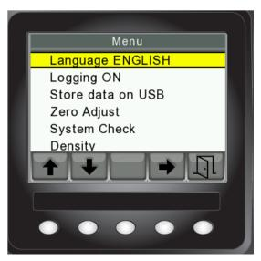
If your moisture meter is installed and prepared by the dealer, you can always go through the menu under the different menu items and change settings or repeat e.g. Zero Adjustment.
