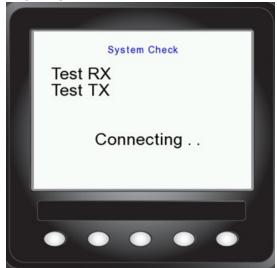
When power is applied to **the display** for the first time, the unit will perform a "system check" and try to contact the RX and TX units.
